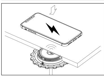
Option 2 - Use adhesive EPDM rubber and align with magnet tool provided. Use Alcohol wipe to ensure surface is free from dirt or grease.
